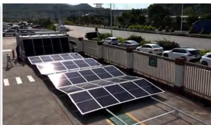
5. Start the winch/motor, deploy the panels.
