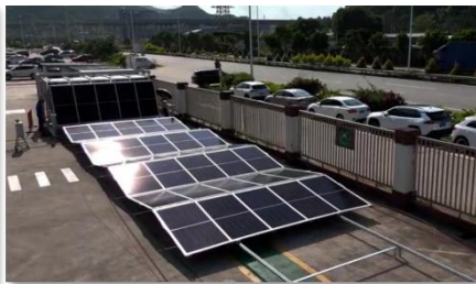
5. Start the winch/motor, deploy the panels.
